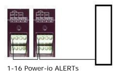
A standard PLC input card where the input is set to PULL UP. Power-io's ALERT output will pull down when an ALERT condition happens. Some PLCs will call the ALERT output a "PLC sinking input signal".
