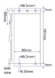
For surface mounting installations: drill and tap for # 10 screws
