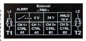
The upper 4 position terminal block is used for the external 24 VDC power supply connection, using screw terminals 2 and 3. The power supply powers the fan and Alert diagnostics. The fan is activated by an internal temperature measurement circuit, as needed. In case of thermal overload, the inputs will be disabled and a red LED will illuminate until the condition is corrected.
