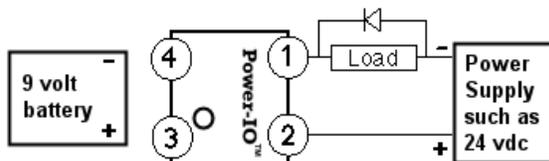
control input is present, load is "on"
